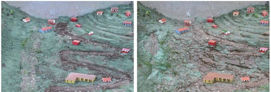
Figure 2-49: Landslide Demonstrator helped people to understand the process of slope movement in their localities, thereby enhancing their involvement in decision making for environmental protection (left photo: 3D model of hillslope with shear failure; Right photo: same terrain after rainfall. Image credit: Bijay Krishna Upadhyay, NSET, Nepal).
